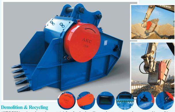
**AKBC 3000** is engineered to crush concrete (reinforced) and rocks and have a robust structure to endure severe working conditions. Full body is made with Hardox and high anti-wearing steel and structure is designed to maximize crushing efficiency at best. Input gate is designed to accept crushing material in max. and output exit is made to produce final crushed debris to a set size by adjuster.
