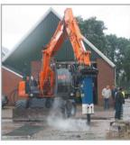
The main points is valve and cylinder adjusters to change frequency according to demolition work conditions.
